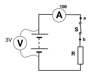
The switch S is then **opened**. The voltmeter across the battery still reads 3V.
