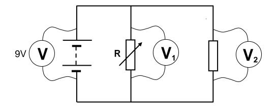
The resistance of the variable resistor, R, is **increased**.
