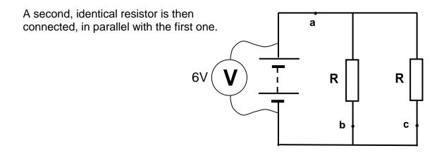
The reading on the voltmeter is still 6V.
